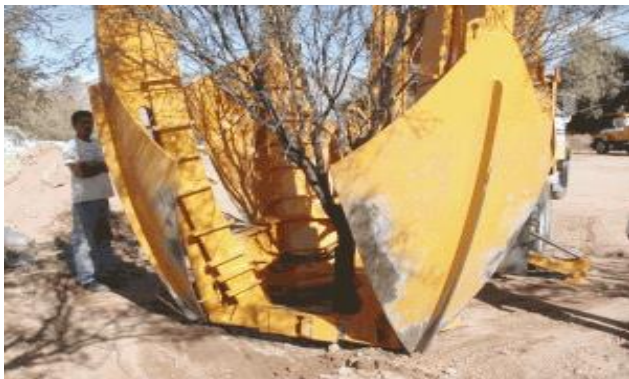
The gate is the closed and locked hydraulically and the entire unit is lowered to the ground
