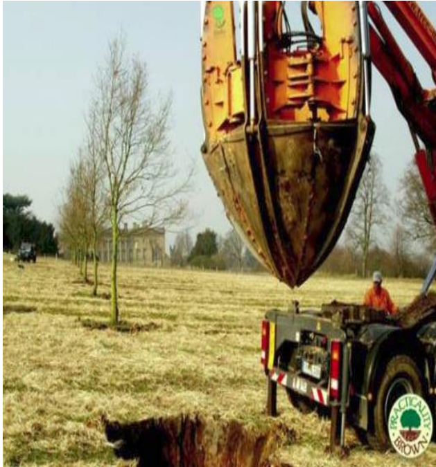
The tree transplanted is first used to dig the first pit at the recipient location
