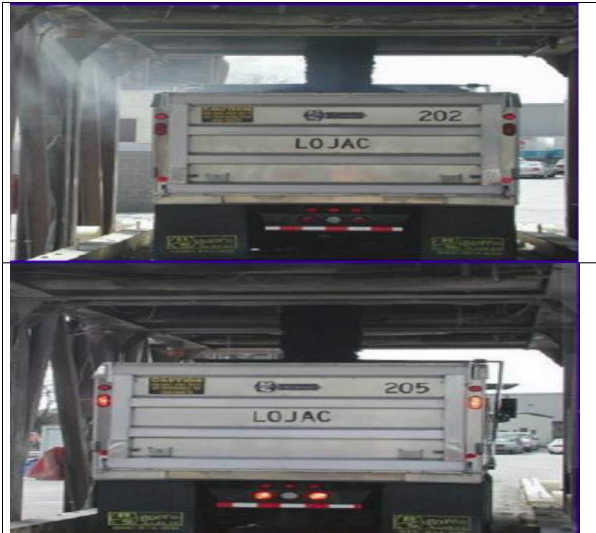
Figure 4.3: Visible Emissions From HMA (Left) In Comparison To WMA (Right)
