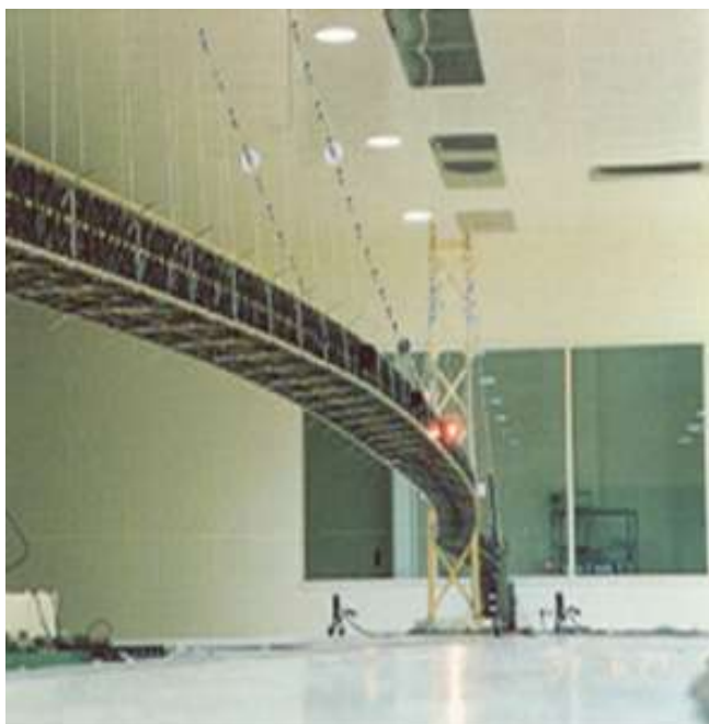
Figure7: 1/100 scale Wind Tunnel model of the Approximately 4 Km long Akashi Kaikyo Bridge.
