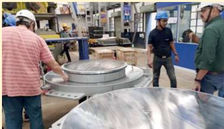
RESTON®PENDULUM DUPLO FPBs being inspected at workshop
